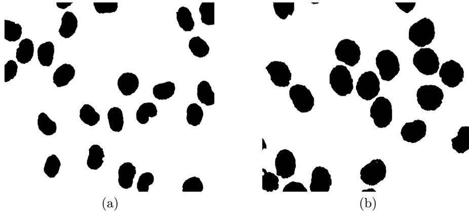
**Fig. 1** The data – cross-sections of heat-treated (a) and untreated (b) carbon fibers.
